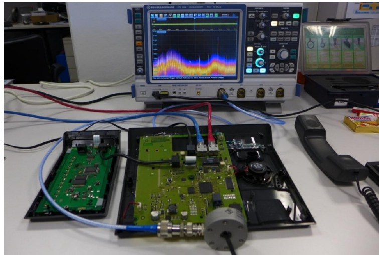
Fig. 4-13: RFI current measurement on the handset line.
