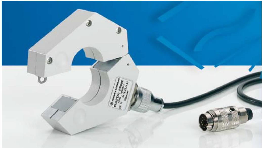
Fig. 3-3: The R&S®EZ-17 current probe with 10 dBΩ transfer impedance (model 02) or 17 dBΩ transfer impedance (model 03) and 20 Hz to 100 MHz bandwidth is a good example of a device suitable for measuring RFI currents. The large inner diameter of 30 mm allows measurements on cable bundles.
